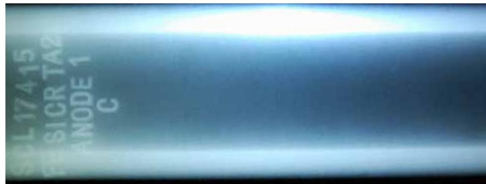
Straight Wall Centrifugally-cast Anode, showing no visible defects. Therefore, better than Level 1 X-Ray.
